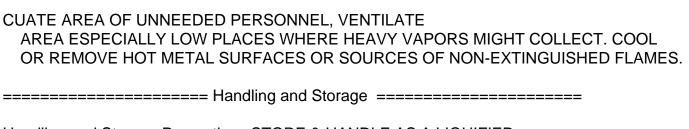
Handling and Storage Precautions:STORE & HANDLE AS A LIQUIFIED COMPRESSED GAS IN DOT' APPROVED PRESSURE VESSELS AWAY FROM HI-TEMPERATURES.
