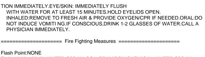
Extinguishing Media: WATER SPRAY, CO2, FOAM/DRY CHEMICAL. WATER SPRAY MAY BE USED TO KEEP FIRE EXPOSED CONTAINERS COOL & FLUSH SPILLS
